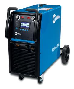
MigMatic® 260i/320i is equipped with a 4-roll wire drive system (2 driven and 2 idle). The rolls are reversible offering flexibility between two different wire sizes. For soft wires, an all-drive system can be supplied as optional extra.
